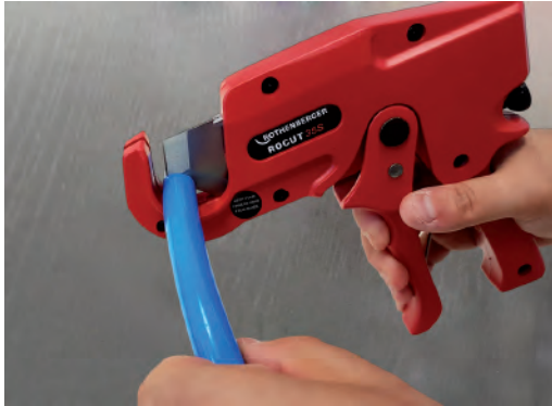
Cut the pipe with the special shear.
